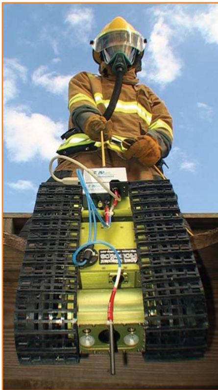
American Standard Robotics in St. Petersburg, Fla., prepares one of their VGTV-Xtreme Reconnaissance Vehicle robots equipped with an Ocean Optics spectrometer to identify the chemical involved in a simulated hazardous-material tanker trailer.
